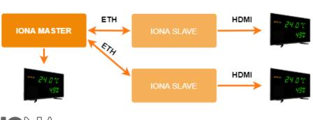
IONA MASTER is an acquisition and display system for measuring ambient temperature and humidity manufactured by **Disenos y Tecnologia**.
